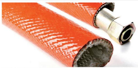
Fire-proof sleeving is fabricated from a dense E-glass fiberglass with a thick coating of self-extinguishing high temperature silicone rubber which is engineered to protect hoses, cables and wire harness from damage due to exposure to extreme heat ,open flame and molten splash.
