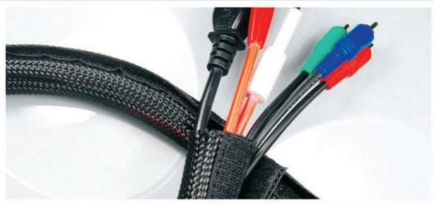
JDD-VCW Velcro braided wrap can help to create a tidy and well-regulated environment. It can be easily wrapped and closed over the cables. It can be re-opened rapidly to manage cables to be added or removed, and breakouts can be made simply by bringing cables out through Velcro. Open weave design easily conforms to many irregular shapes.
