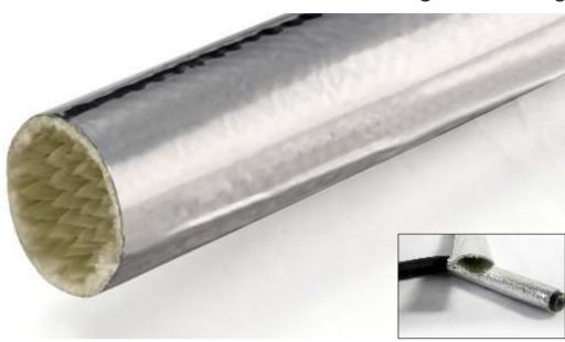
AFR1067 aluminum heat reflect fiberglass sleeving is special designed by laminating an aluminized metallic heat shield to a layer of strong and tight braided fiberglass yarn. A special manufacturing process permits the sleeve to boast a virtually seamless and non fraying construction. This aluminized fiberglass sleeve reflects more than 95% of the radiant energy that hits its surface, keeping the underlying cables, hoses and wires cool.
